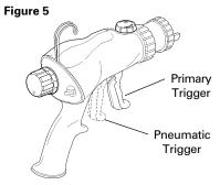
For Primary Trigger Use - rotate trigger foreward approximately 20° and pull downward.
