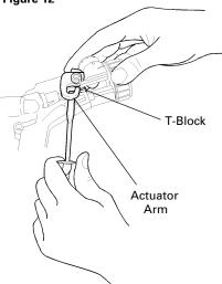
4. To remove actuator (22), wedge a screwdriver between the actuator and horn air valve (see Figure 13). Then, using a pencil or similar tool, pry the actuator back off the skeleton mounting posts as shown.
