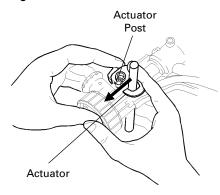
6. To assemble T-block (23) into actuator, the rounded end must be facing forward, Figure 15, toward the spray head. Install T-block into gun body slot in front of actuator with flat edge into the actuator. Use a small screwdriver to push T-block through into actuator arm on opposite side, Figure 16. At that point, flex actuator arm ear out past T-block and push T-block fully into actuator arm, Figure 17.
