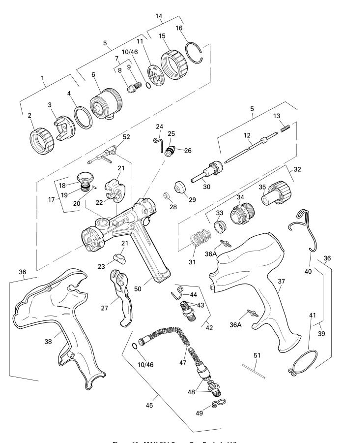
Figure 10 - MAX-504 Spray Gun Exploded View
