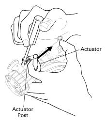
5. Install the new actuator (22) onto the skeleton as shown in Figure 14.
